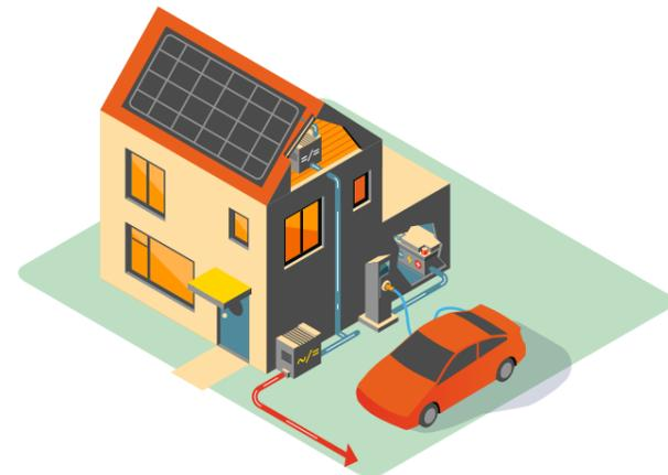
Figure 1 Local DC voltage micro-grid with smart combination of solar PV and V2G
