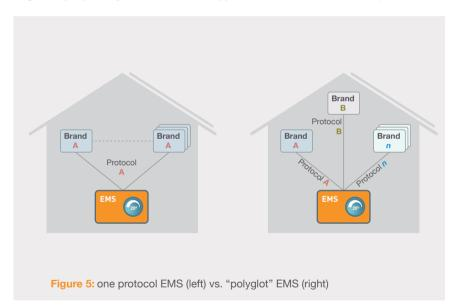
Following this approach it is possible to send detailed information to the flexible device itself. For example, an EMS can use energy prices to optimize the charging plan of an EV, by sending maximum power limit signals to the charging station. When using multiple devices such as solar panels, heat pumps, charging stations, the EMS takes care of optimization and sending signals to each of the devices.
