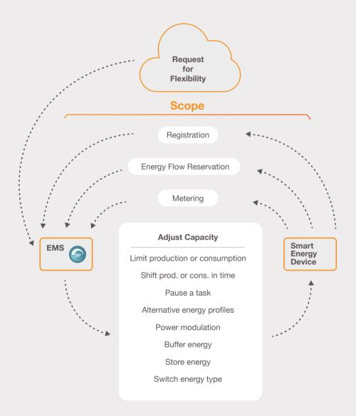
The function Adjust capacity can thus be used to communicate different flexibility patterns. Depending on the chosen architecture (next chapter) these patterns can be implemented in the EMS, the smart energy device or in an adaptor/convertor module between the EMS and the flexible device. In the next chapter this will elaborated on.
