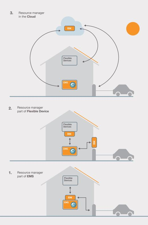
When applying this architecture the consumer can still control and influence the operation of 'in-home' flexible devices and determine the amount of energy flexibility. The consumer probably has its own set of preferences for the behavior of their flexible device that must be taken into account by the EMS. These preferences shall take precedence over those of the energy stakeholders unless otherwise specified.
