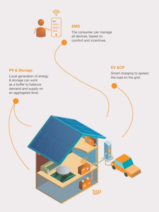
A dense installation of solar panels in a neighborhood cause peaks in local electricity generation, electric cars cause a simultaneous and substantial power demand. And other devices, such as heat pumps and inductive cooking, can also cause a simultaneous peak demand. However, many of these devices also offer control possibilities; unlocking flexibility from these devices.
