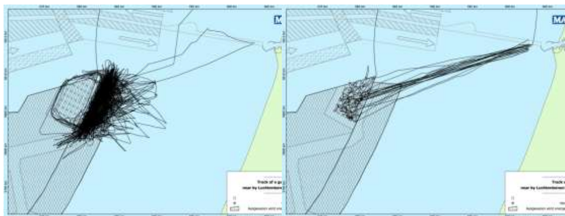
Figure 4-11 Track of different type of work vessels in different operational phases of the wind farm Luchterduinen.
