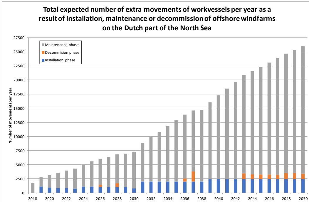
Figure 5-1 Total expected number of extra movements/visits of work vessels per year as a result of installation, maintenance or decommissioning of offshore wind farms on the Dutch part of the North Sea.
