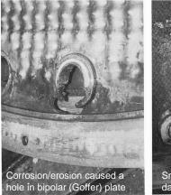
Fig 4 Perforated goffer plate
